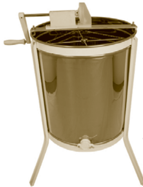
4 Frame Extractor Tangential
